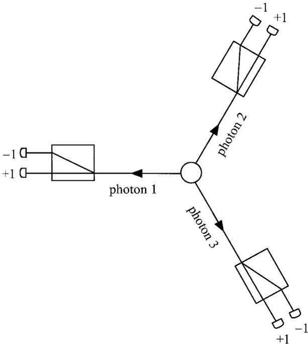
**Figure 6** The apparatus used in the Greenberger–Horne–Zeilinger argument. Three photons prepared in a particular state are emitted from the source. Measurements of polarization are made on each photon with the corresponding calcite crystal orientated either at  $0^\circ$  or  $45^\circ$ .
